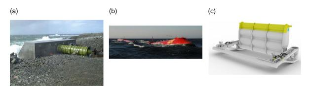
Figure A6. In-grid WEC technologies developed in the UK. (a) LIMPET OWC installed on the island of Islay, Scotland, rated 500 kW [24] (b) Pelamis [32] (c) Oyster 800 [33].
