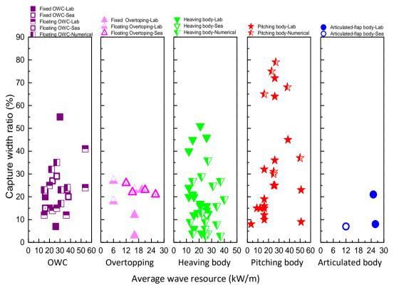
Figure C2. Capture width ratios of WECs as a function of wave resource with respect to different working principles.
