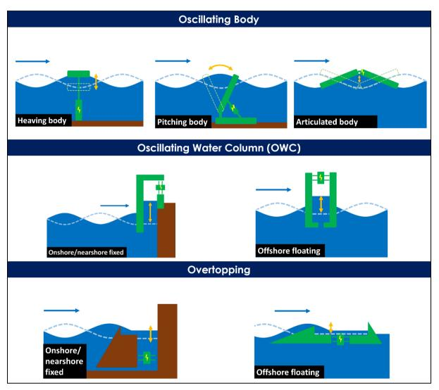
Figure 2. Categories of WEC technologies by operating principles
