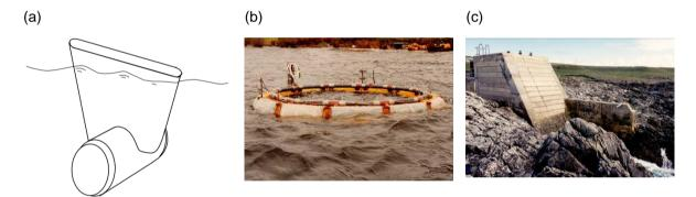
Figure A5. Early WEC technologies developed in the UK. (a) PS Frog [31] (b) Circular SEA Clam [29] (c) Shoreline OWC on the island of Islay, Scotland [24].
