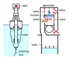
Figure B1. Layout of Masuda's navigation buoy
