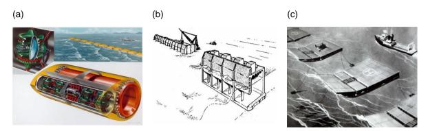
Figure A4. Representative WEC technologies supported by the British wave energy programme 1974–1983. (a) Edinburgh's Duck [28] (b) NEL OWC [24] (c) Cockerell Raft [30].
