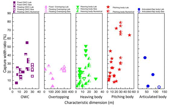
Figure C1. Capture width ratios of WECs as a function of characteristic dimension with respect to different working principles.
