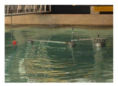
Figure A9. M4 WavePower from University of Manchester [35]
