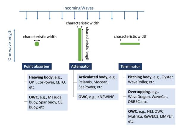
Figure 3. Categories of WEC technologies based on their orientation and the sub-categories with respect to working principle.
