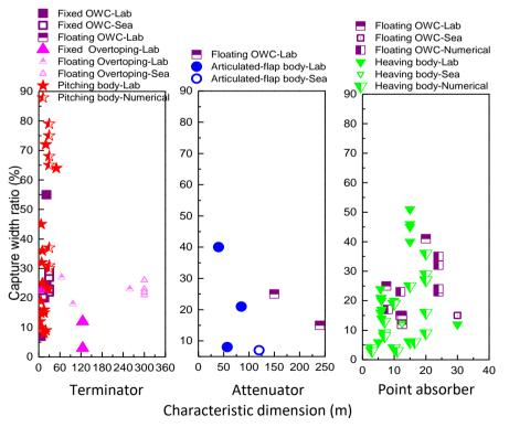
Figure C3. Capture width ratios of WECs as a function of characteristic dimension with respect to different WEC orientation.
