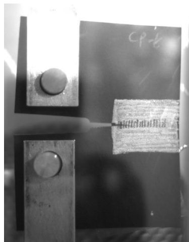
Figure 1. The compact tension test specimen captured by the video gauge set up.
