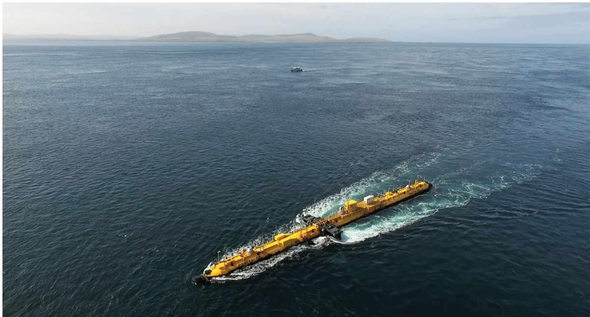
Figure 1 The O2 floating tidal turbine (Orbital Marine Power) with our survey boat, the Green Quest in the background.
