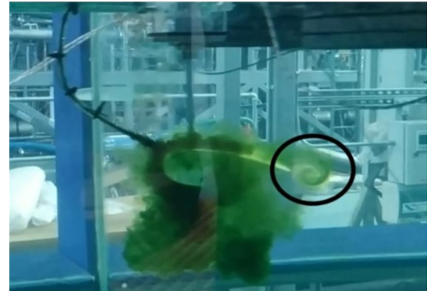
Figure 3: Flow visualisation indicating the formation of a Reversed von Karman streets.
