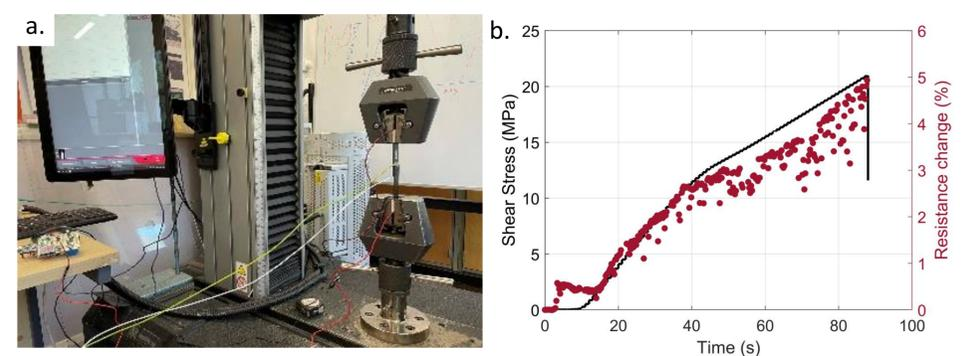
Fig.3 Tensile test setup (a) and representative results of lap shear strength (b)
