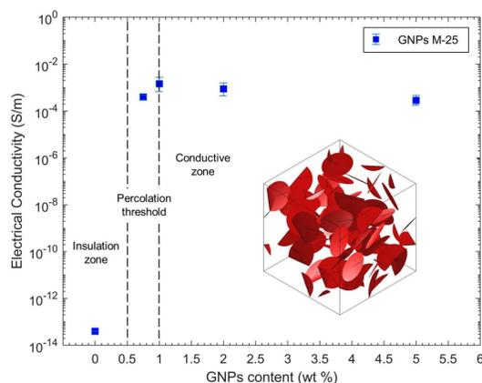
Fig.1 Electrical conductivity versus GNPs loading
