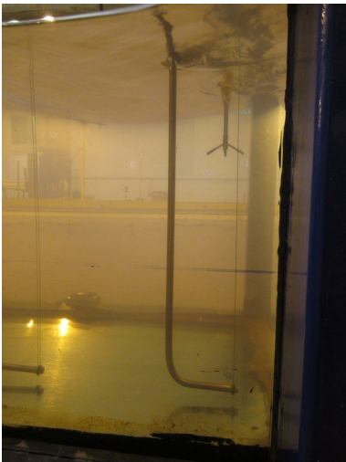
Figure 1: Lateral view on the Nortek Vectrino Profiler and wave probe
