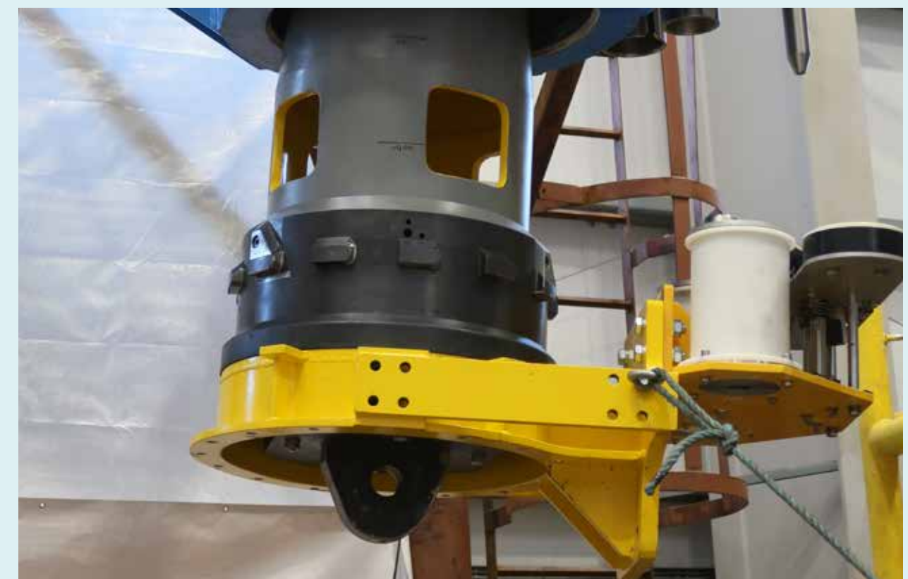
Quocean's Q-Connect quick connection system (Credit: Quocean)
