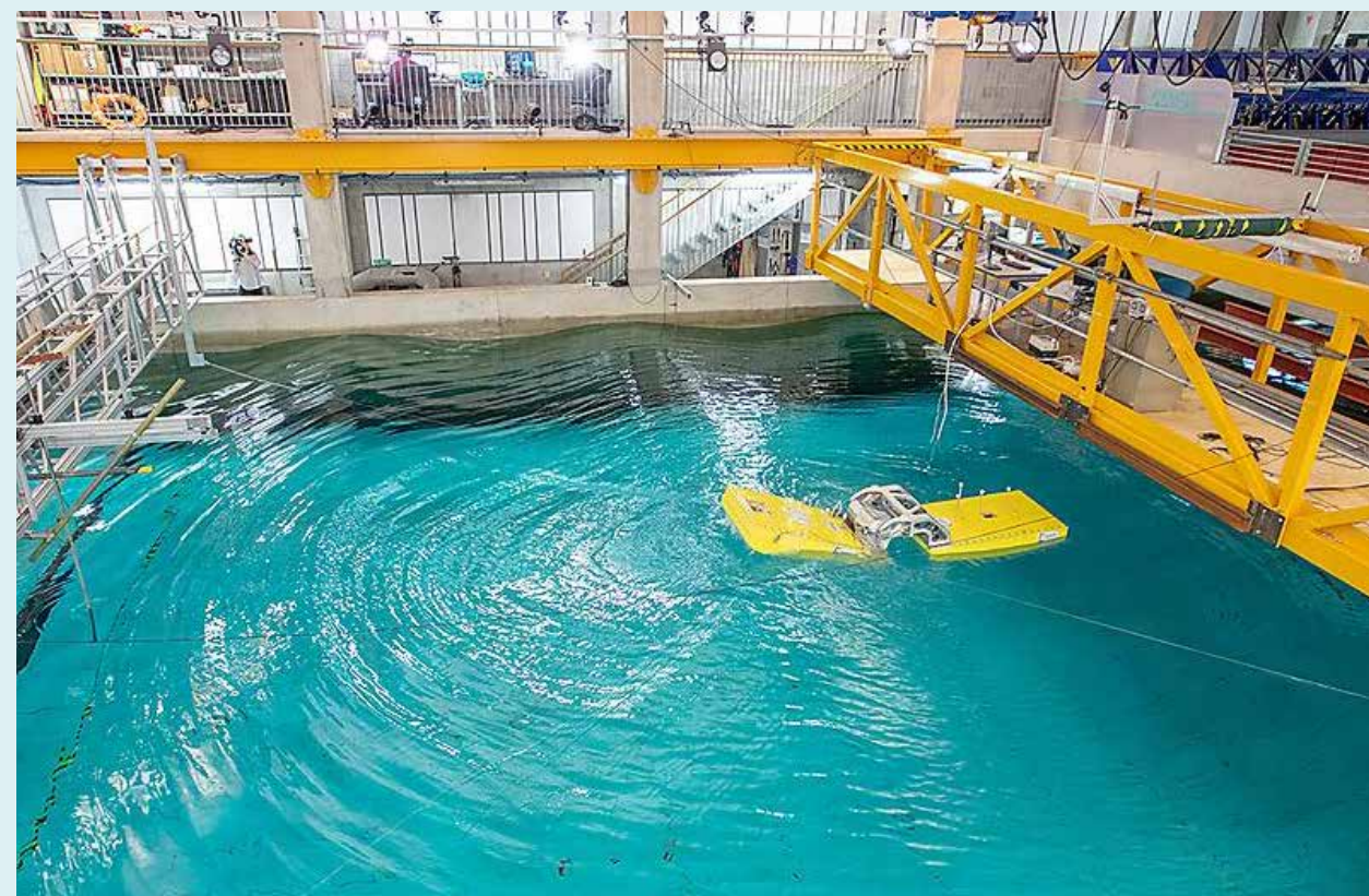
Tank testing at University of Plymouth's COAST Lab (Credit: University of Plymouth)
