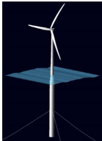
Figure 2-1 Hywind spar with NREL 5MW turbine. Example data is illustrated on the right-hand side.
