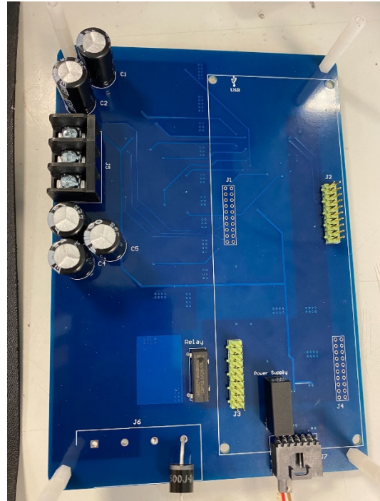
Figure 14: Actual fabricated PCBs with components partially populated
