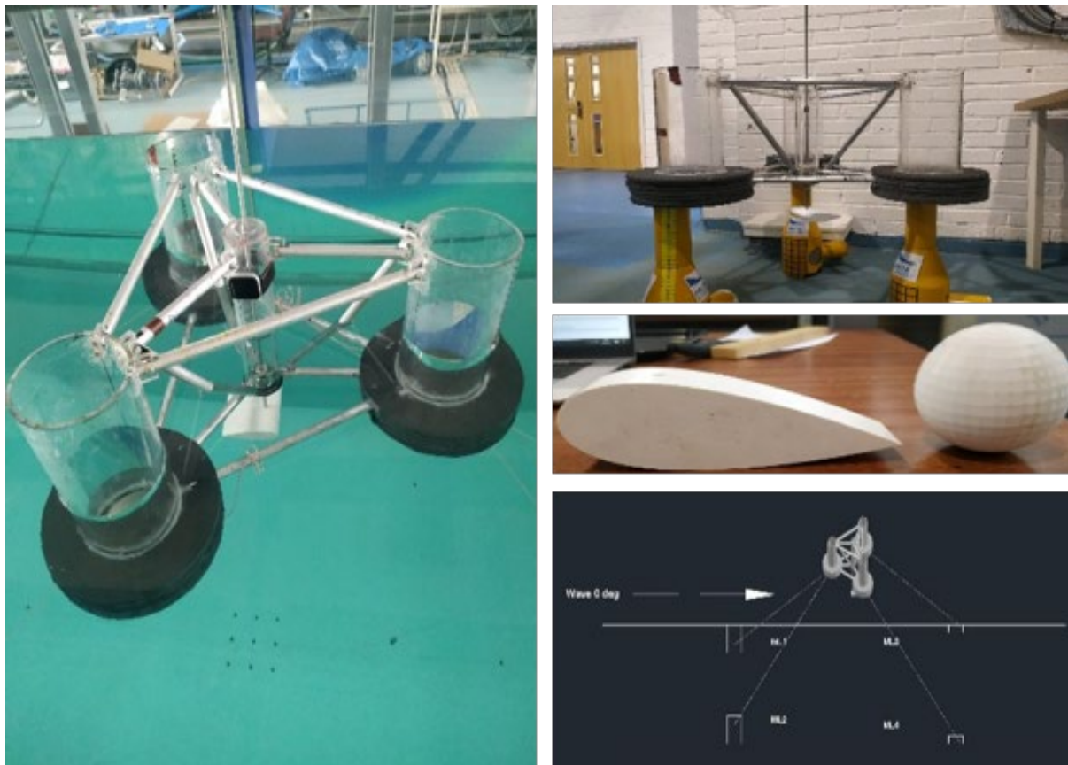
Figure 1: on the left, the model platform in the wave flume. At the top right, photograph of the model equipped with a hydrofoil. Below, on the tested hydrofoils and the, equivalent volume, sphere. At the bottom right, schematic of the mooring line arrangement used for all the tests.
