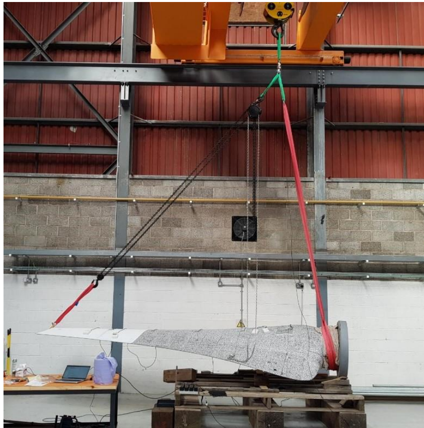
Figure 5 - Blade weight and centre of gravity measurements
