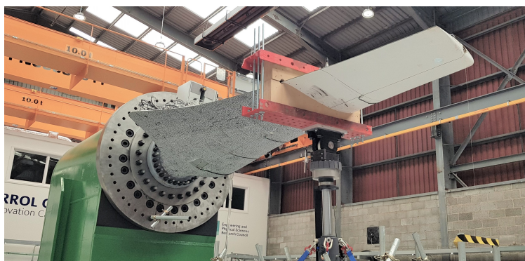
Figure 4.6: MDF fitted load introduction system
