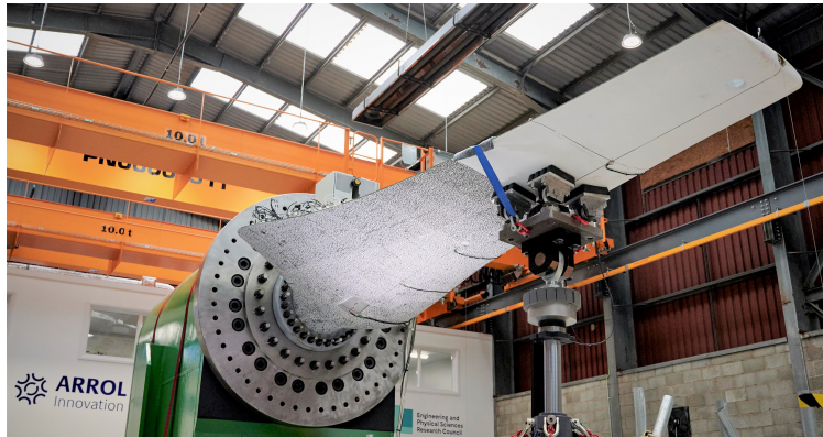
Figure 4.5: Articulated pad, load introduction system
