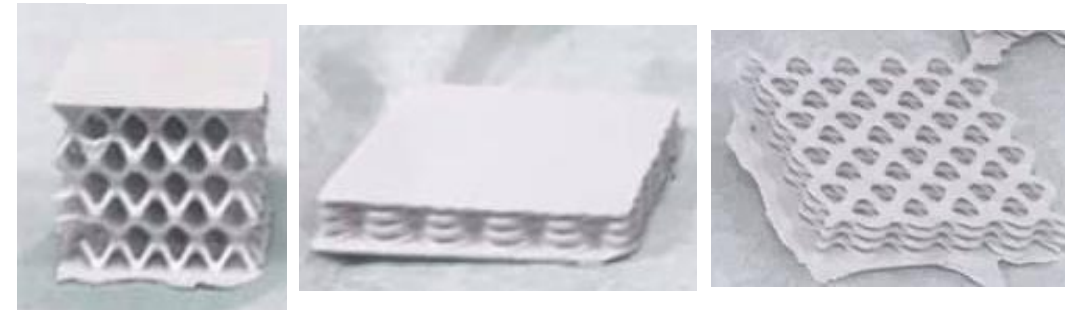
Printed structures made with a polymer piezoelectric particle nano-composite.
