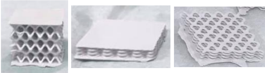
Figure 2: Printed structures made with a polymer piezoelectric particle nano-composite.
