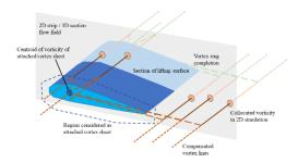
Illustration of the proposed correction to 2D strip theory models using vortex rings
