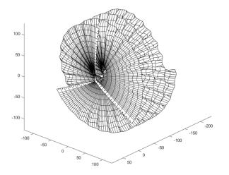
Far-field wake behind a wind turbine. Not visible is a near-field model consisting of a 2D vortex panel model with partial dynamic flow separation.
