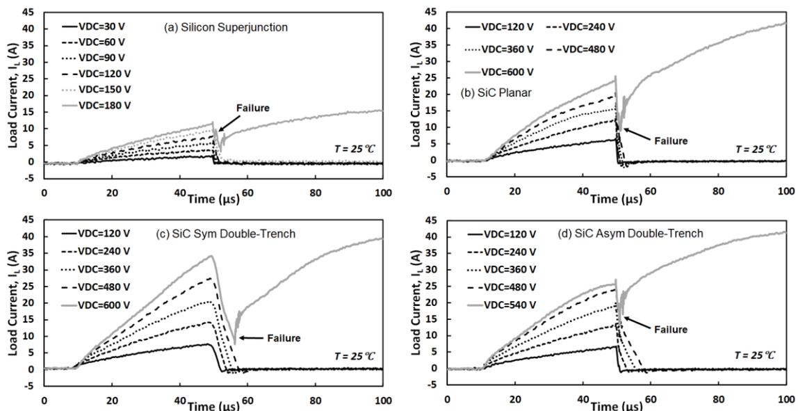
Fig. 3. Avalanche load current of the four devices for various DC-link voltage until the devices failed at 25°C.
