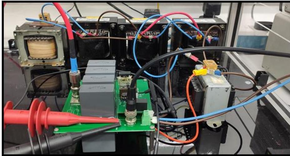
Fig. 2. Experimental test setup of the Unclamped inductive switching test board.
