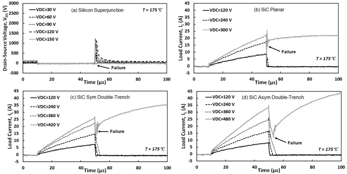
Fig. 4. Avalanche load current of the four devices for various DC-link voltage until the devices failed at 175°C.
