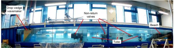
The experimental set up was replicated numerically in CFD to compare the results and see if the numerical model could be used for future design optimisation.
