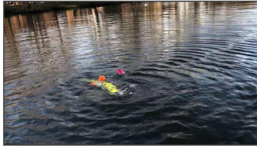
Initial functionality trial at Uni of York lake; body is watertight & actuating with slow propulsion
