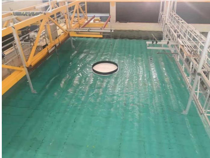
Fig. 7. Regular waves interaction with the floating elastic disk in the Ocean Basin. Obvious wave scattering is observed.
