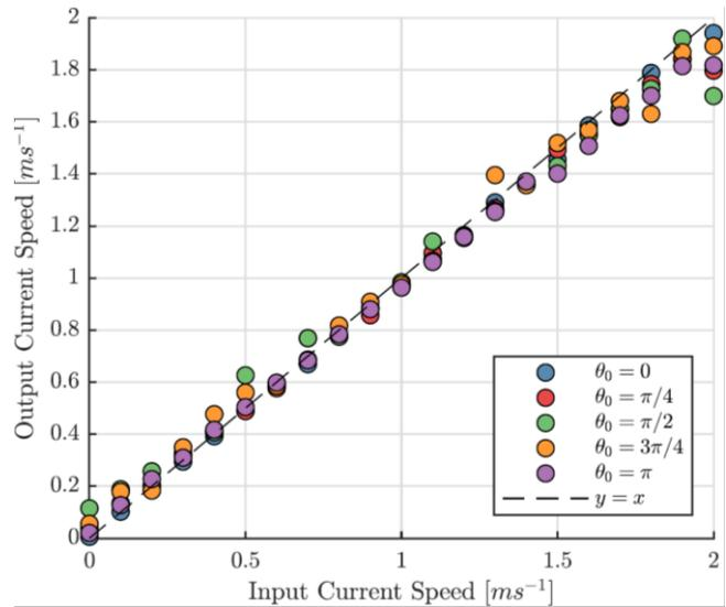
**A Mesh Adaptive Direct Search (MADS) algorithm was used to analyse simulated wave-current buoy data, solving for unknown wave and current parameters. It proved capable of resolving complex bimodal spectra, and highly effective at extracting the underlying current velocity at different relative wave-current angles (the input (simulated) vs. output (MADS) speeds shown in plot).**
