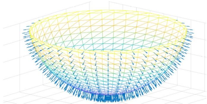
**Wave buoy behaviour in wave-current sea states was modelled both physically in the FloWave test facility, and numerically using a frequency domain model, with hydrodynamic coefficients obtained through the open source NEMOH Boundary Element Method (BEM) package.**
