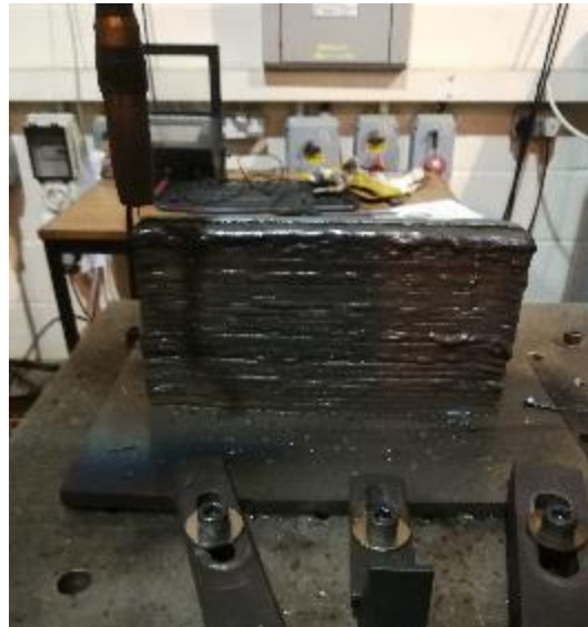
Figure 1: An example of a WAAM wall produced using ER70 steel
