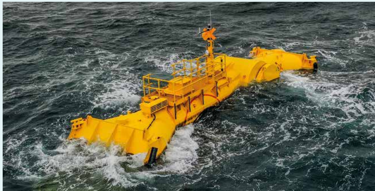
Mocean Energy's Blue X wave energy converter, at EMEC Scaapa Flow test site (credit: Mocean Energy/Colin Keldie)
