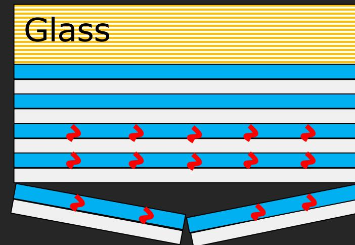
Fragmentation of the inner low strain carbon fibre material
