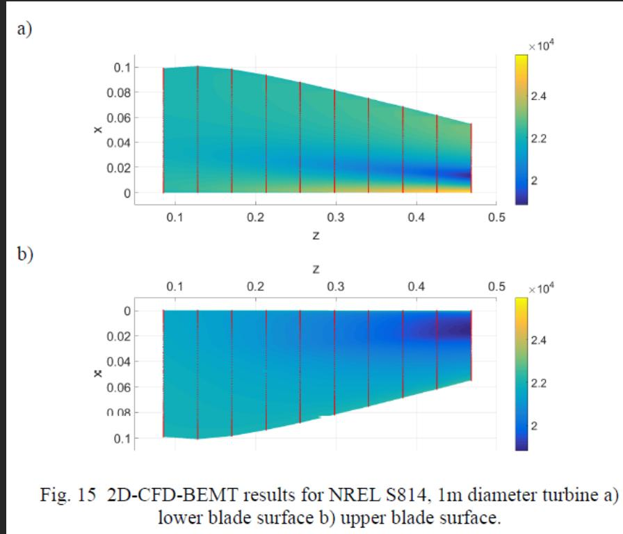
Fig. 15 2D-CFD-BEMT results for NREL S814, 1m diameter turbine a) lower blade surface b) upper blade surface.
