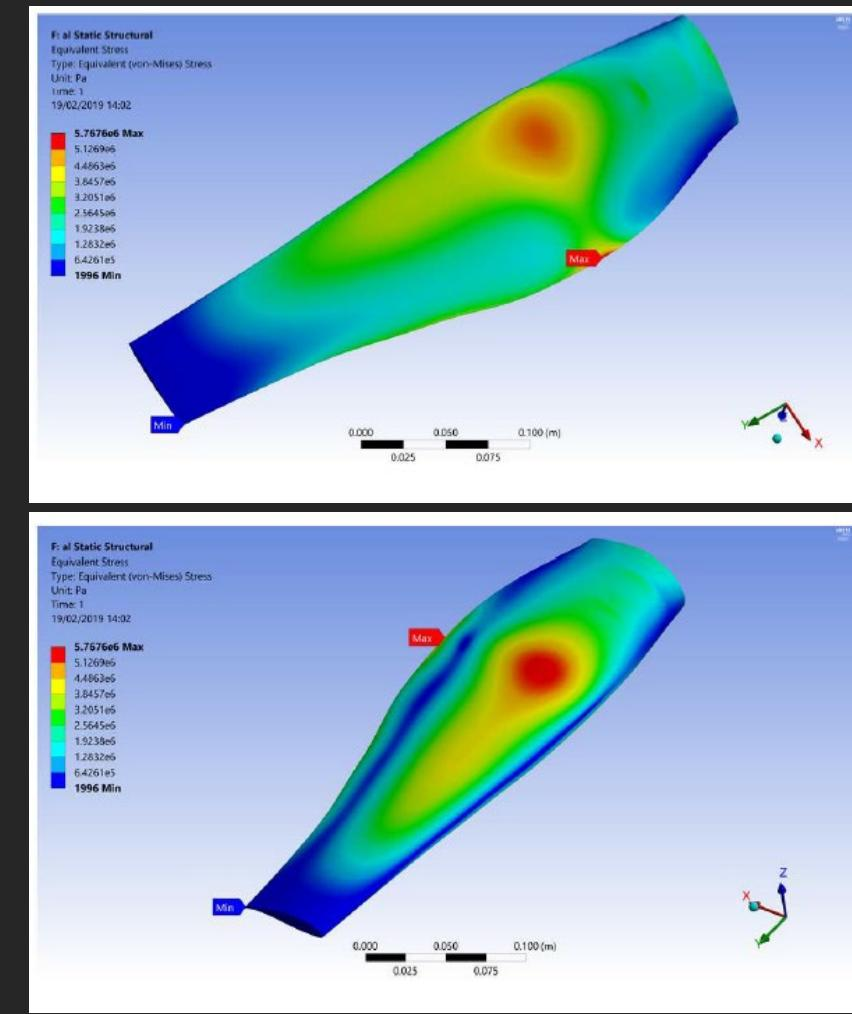
Assessment of loadings for a thermoplastic tidal stream turbine blade using ANSYS.
