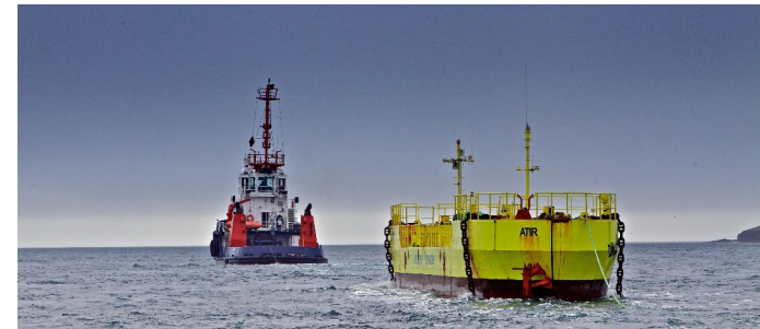
1.5MW floating tidal turbine – Summer '21
