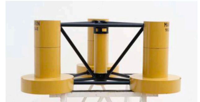
DeepCwind Semi-submersible floater
