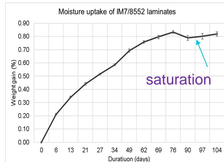
“wet” specimens conditioned at 70 °C and 85% relative humidity
