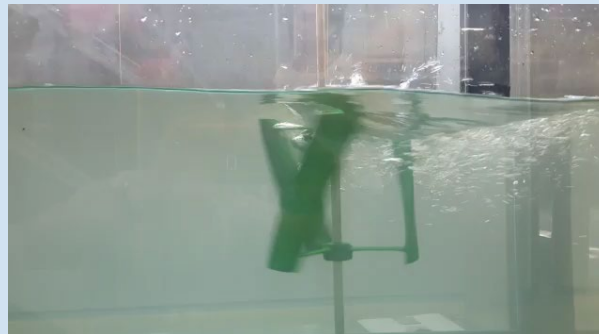
Vertical axis turbine with a helix shape for low velocities (IIUNAM)
