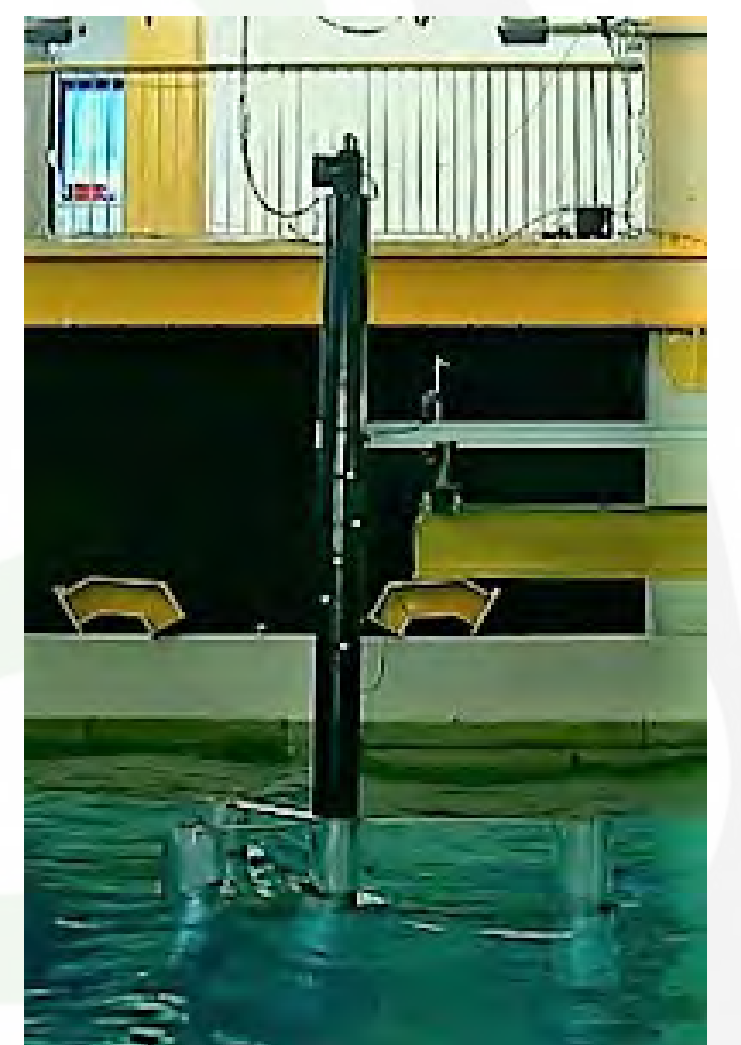
Figure 4: Photograph of the COAST Lab's 1:70 scale model of the VoltturnUS-S 3 .
