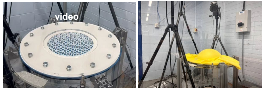
Bulge test for new material
