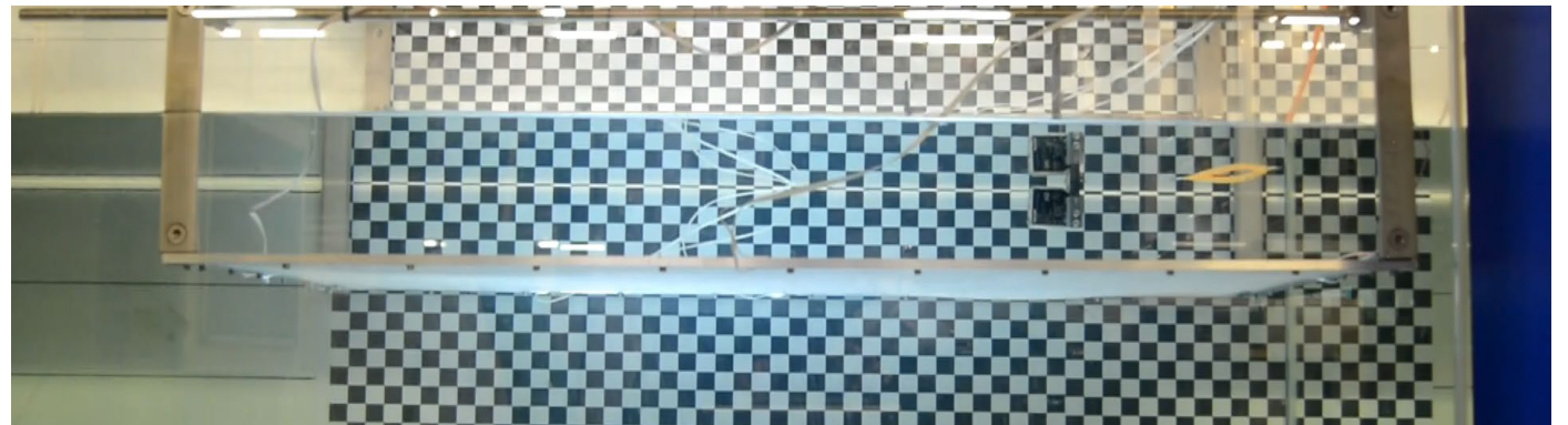
Interaction of Silicone membrane with regular wave
