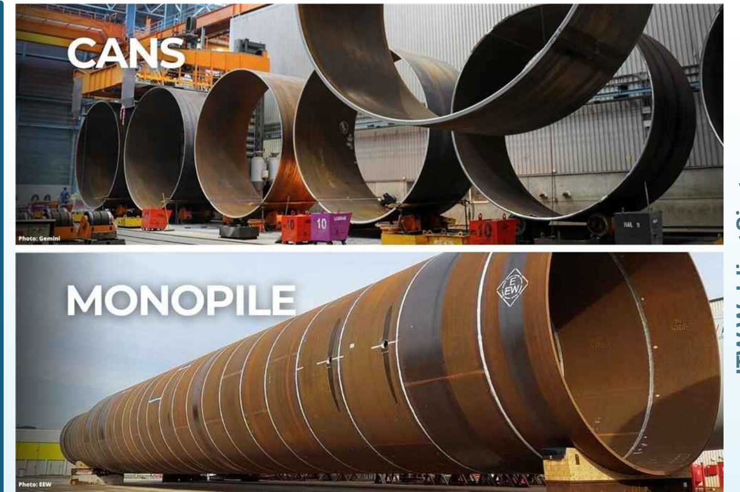
ITW Welding Singapore The Welding of Offshore Wind Monopiles
