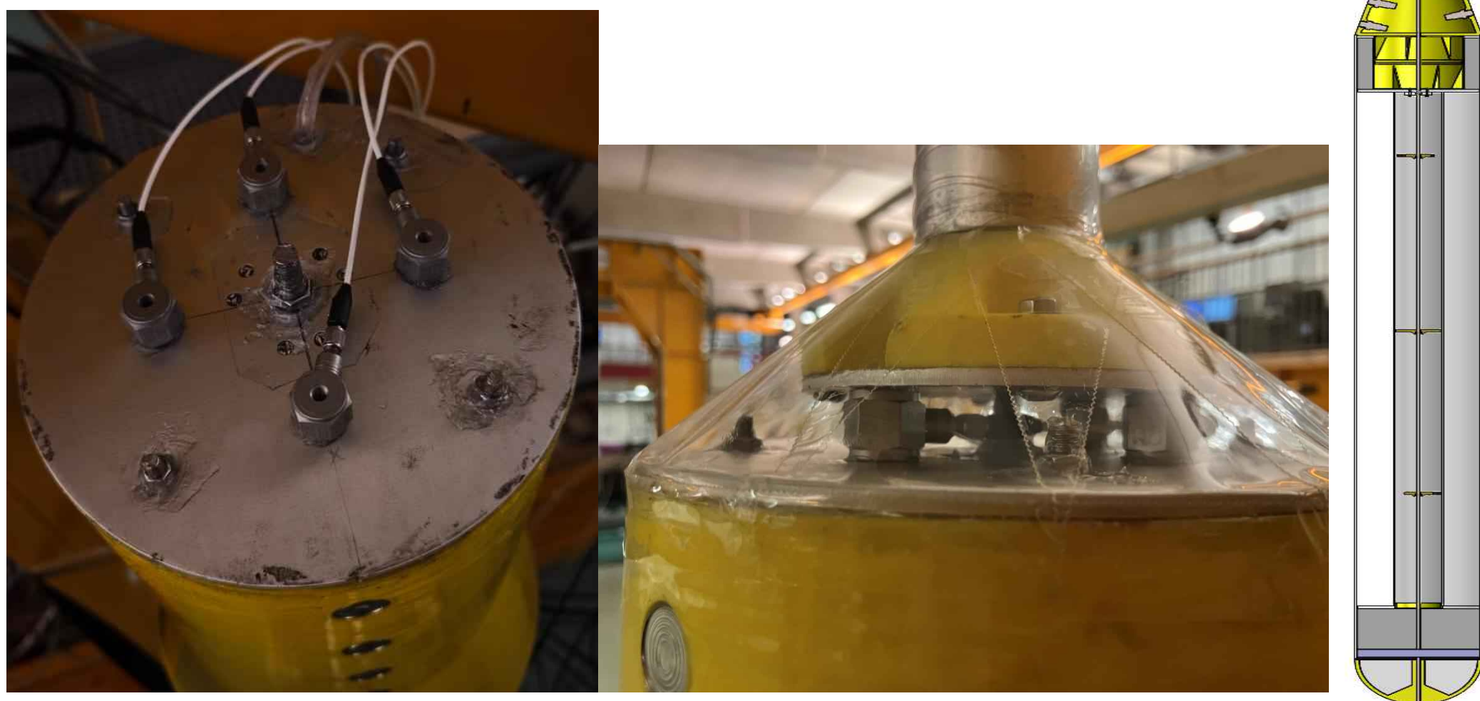
Fig.1 (left to right) Single axis load cell arrangement used to calculate tower base bending moments, deployed load cells at tower base, CAD model of fully assembled model.
