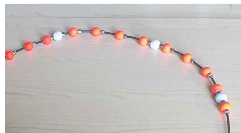
Model of the future Commercial Scale Demonstrator at scale 1:62, semi-submersible platform with heave plates
